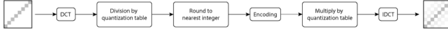
Figure 4.7: A typical quantization process converts an image to its DCT coefficients, normalizes the values using a quantization table and rounds the values. The encoding is imperfectly reconstructed by reversing the normalization and domain transform.
